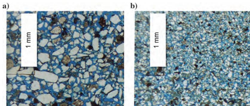
**Figure 3.** Thin sections describing pore network systems (HRT) formed by different grain sizes. (a) HRT-1 (porosity = 32 p.u., permeability = 852 mD); (b) HRT-3 (porosity = 27 p.u., permeability = 121 mD).
