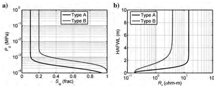
**Figure 5.** (a) Drainage capillary pressure, and (b) resistivity-height relation of two different rock types. Here,  $P_c$  is capillary pressure; HAFWL is height above free water level; and  $R_t$  is resistivity.
