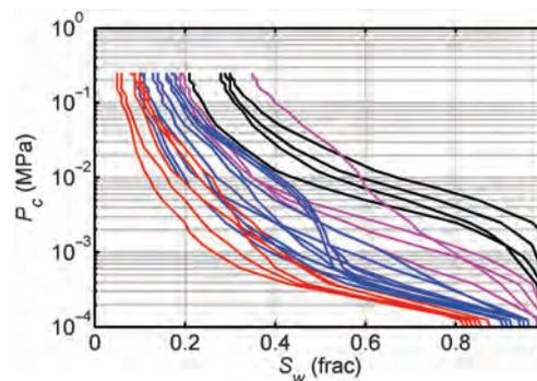
**Figure 8.** Primary drainage capillary pressure curves modeled from laser particle size analyzer measured grain-size distributions.
