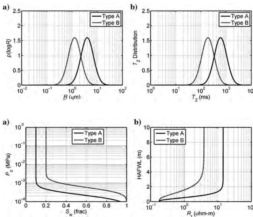
**Figure 4.** (a) Pore-size distributions, and (b) NMR  $T_2$ -distributions of two different rock types exhibiting different grain-size distributions.
