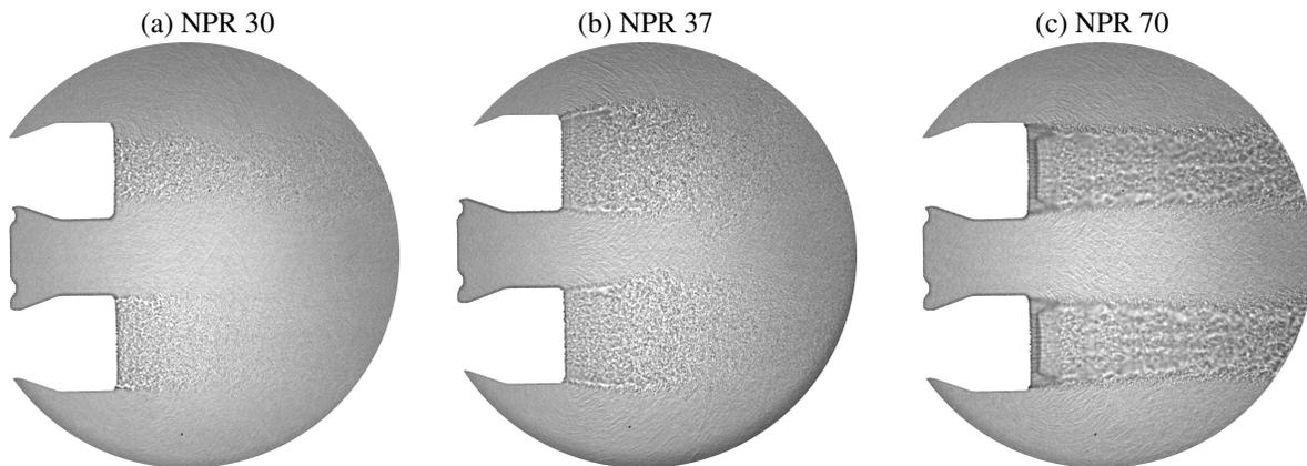
**Figure 2.** Shadowgraphy images of the instantaneous rocket plumes during non-stationary start-up at (a) 30, (b) 37, (c) 70.
