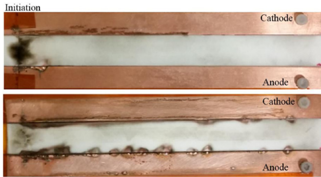
Figure 7. Comparison of electrode topologies after the first firing (top) and the fifth firing (bottom). Notice the continuous damage on the cathode side and the spot damage on the anode side.
