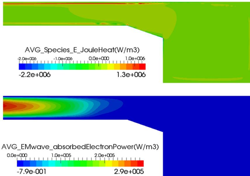
**Figure 4.** Computational results for the electron power deposition in the reactor for 100 mTorr argon discharge driven at 60 MHz. Top: electrostatic Joule heating in the plasma-electrostatics only case. Bottom: EM power deposition in the coupled plasma-EM wave case.
