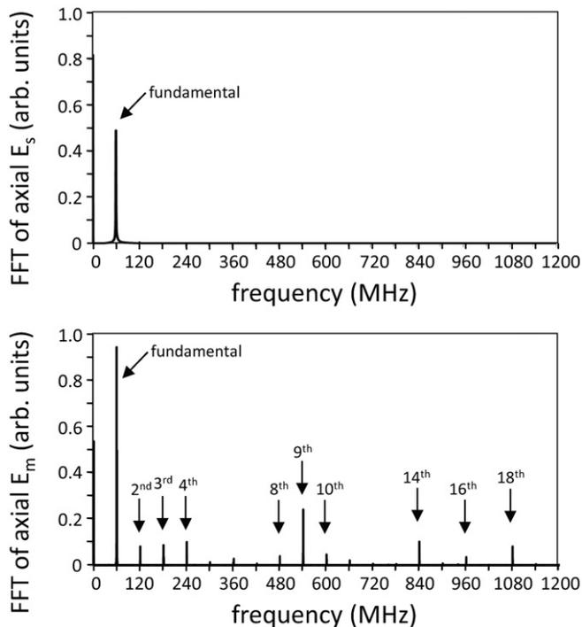
**Figure 5.** FFT of the axial electric fields in the mid-gap axial location of the reactor for 100 mTorr argon discharge driven at 60 MHz. Top: FFT of the electrostatic field in the plasma-electrostatics only. Bottom: FFT of the EM field in the coupled plasma-EM wave case.
