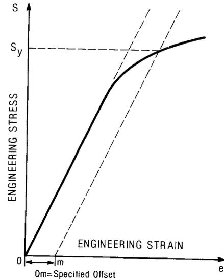
FIG. 4 Stress-Strain Diagram for Determination of Yield Strength by the Offset Method
