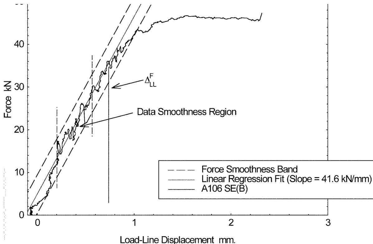
FIG. A14.7 Force Smoothness Verification Schematic
