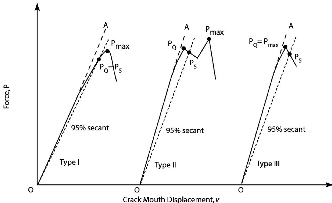
FIG. A5.1 Principal Types of Force-Displacement Records
