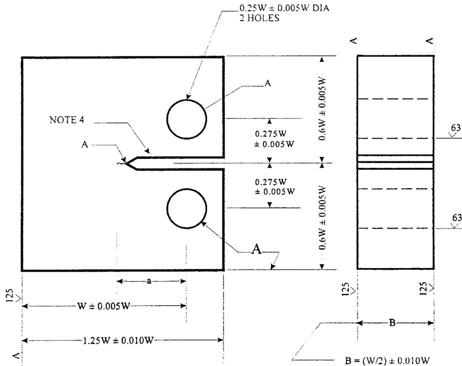
NOTE 1—A surfaces shall be perpendicular and parallel as applicable to within 0.002 W TIR.
