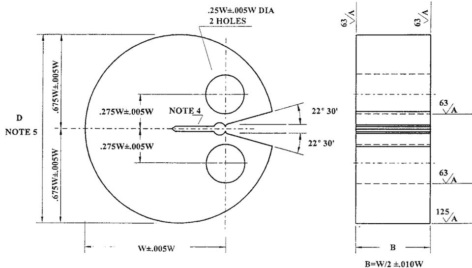
NOTE 1—All surfaces shall be perpendicular and parallel as applicable within 0.002  $W$  TIR.
