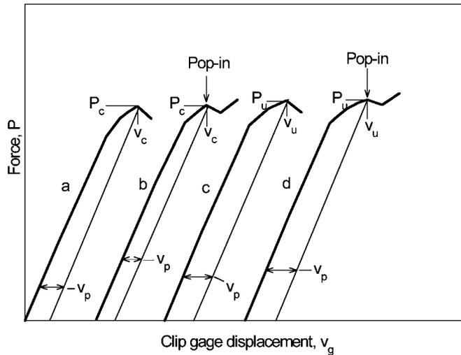
NOTE 1—Construction lines drawn parallel to the elastic loading slope to give  $v_p$ , the plastic component of total displacement,  $v_g$ .
