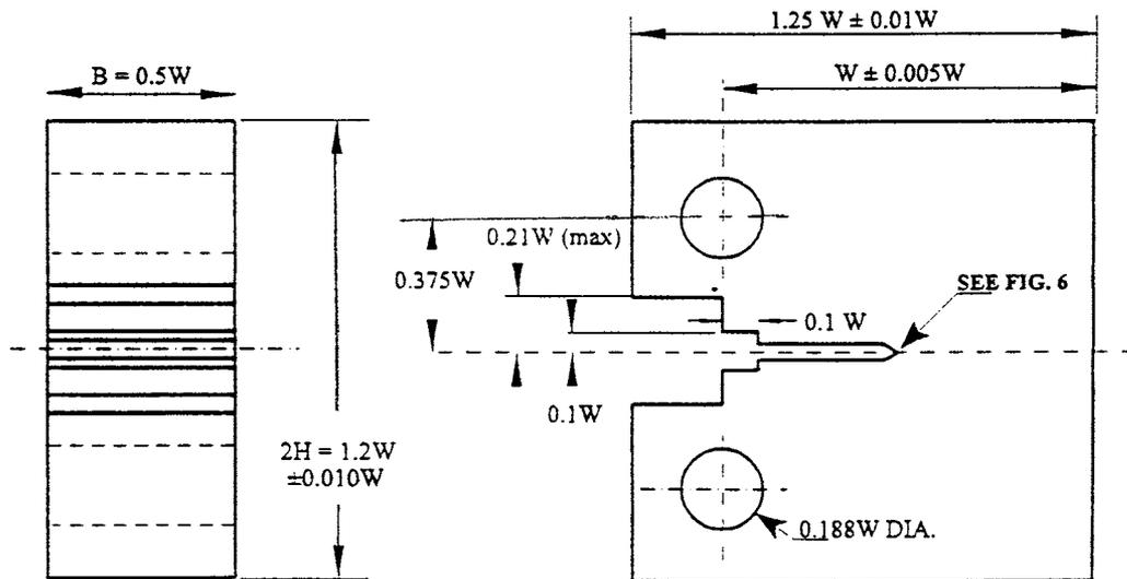
COMPACT TEST SPECIMEN FOR PIN OF 0.1875W(+0.000W/-0.001W)DIAMETER
