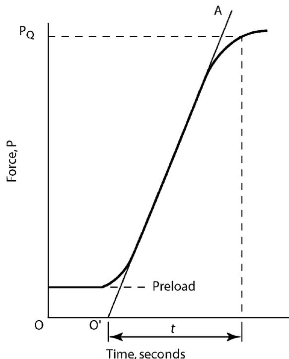
FIG. A13.2 Determination of Test Time from Force versus Time Record
