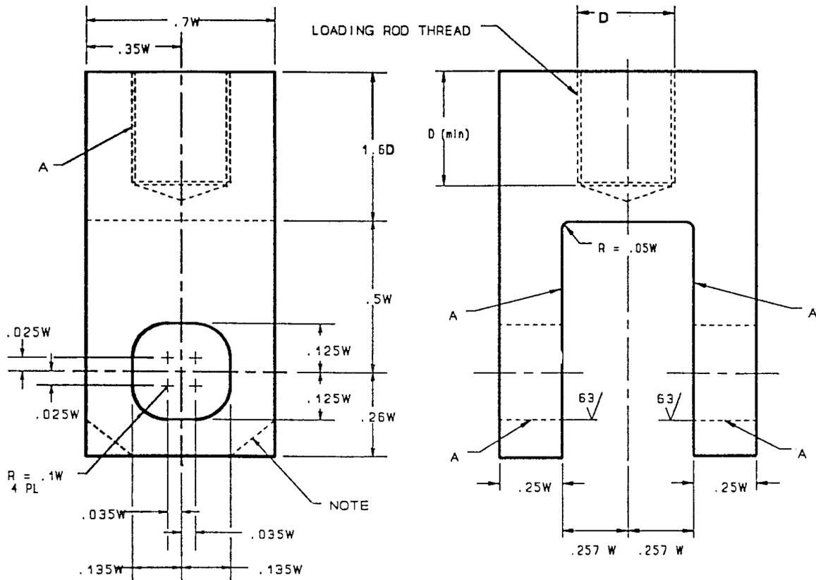
A - SURFACES MUST BE FLAT, IN-LINE AND PERPENDICULAR, AS APPLICABLE, TO WITHIN 0.002 in. T.I.R. (0.05 mm)
